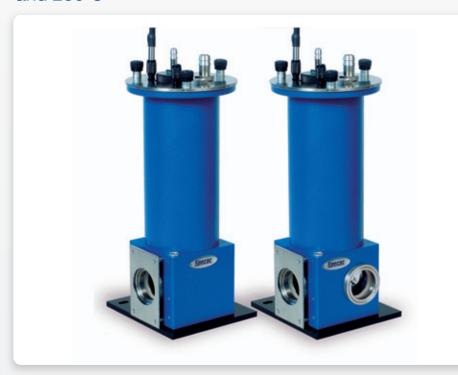
The Variable Temperature Cell Holder is the ideal accessory to use for the transmission study of liquid or solid samples between a temperature range from -190°C and 250°C.
